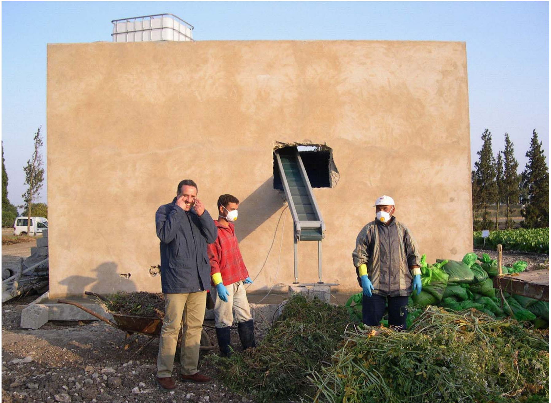
The rear part of the system from where the loading of waste into the bioreactor takes place through a conveyor belt – the waste material (Sludge, green waste, leaves and tree braches) are ready to be fed to the system
